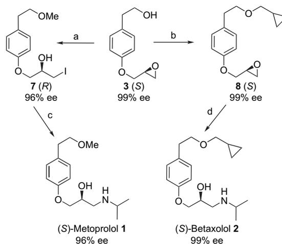
Scheme 3. Reagents and conditions: (a)  $CH_3I$ ,  $KO^tBu$ , *N,N*-dimethylacetamide, 98%; (b) bromomethylcyclopropane,  $KO^tBu$ , *N,N*-dimethylacetamide, 96%; (c) isopropylamine, water, reflux, 97%; (d) isopropylamine, water, reflux, 96%.
